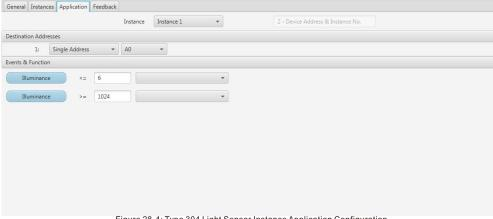
Figure 28-4: Type 304 Light Sensor Instance Application Configuration
