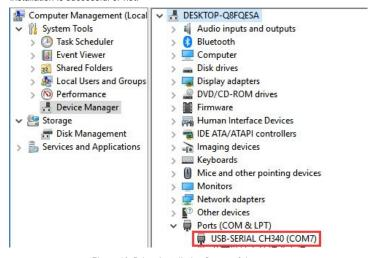
Figure 46: Driver Installation Successful
